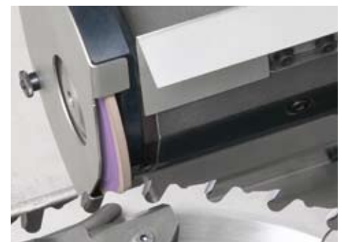
Tool body processing with CBN grinding wheel.
