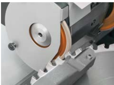
Clearance surface processing with left spindle nose.
