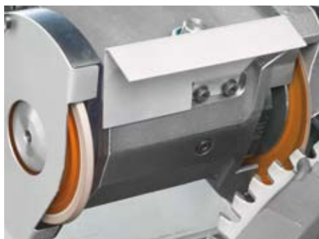
Hook surface processing with right spindle nose.
