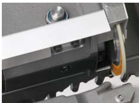
Clearance surface processing with combi grinding wheel.
