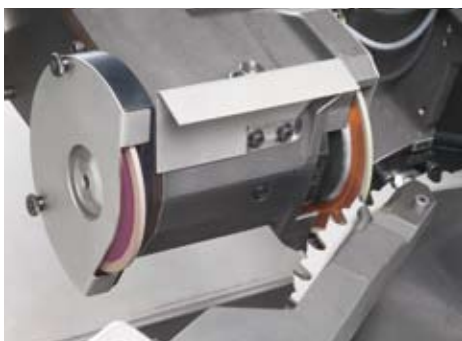
Hook surface processing with combi grinding wheel.
